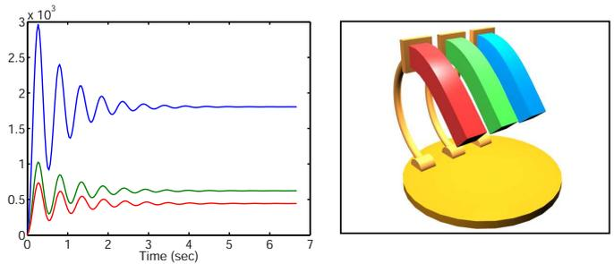
Fig. 11.  $\|\mathbf{R}^T \mathbf{M} - \mathbf{M} \mathbf{R}^T\|$  in three different mesh resolutions:  $11 \times 3 \times 3$  (red),  $19 \times 4 \times 4$  (green), and  $21 \times 5 \times 5$  (blue)
