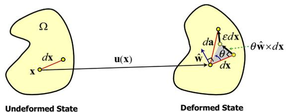
Fig. 1. Kinematics of infinitesimal deformation.
