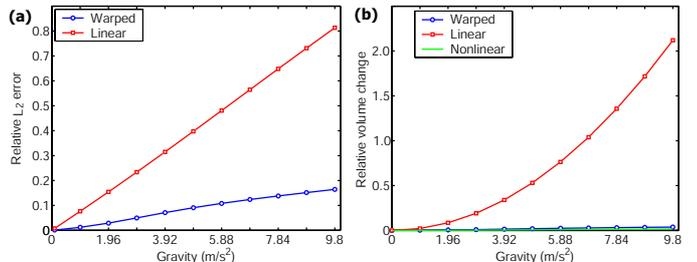
Fig. 5. Error analysis of the bar shown in Fig. 4. (a) the relative  $L_2$  displacement field error and (b) the relative volume change with respect to the initial volume.
