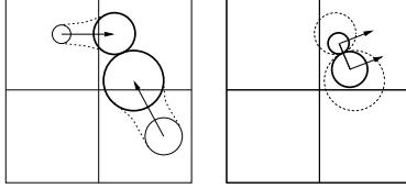
Figure 4: A colliding event for two time-varying bounds (left). A contacting event for two spheres (right).
