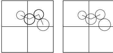
Figure 5: A separating event for two spheres occurs when their relative velocity becomes non-zero (left), and the contact graph is updated (right).
