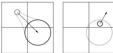
Figure 3: A resetting event occurs when the diameter of a time-varying bound reaches to the length of an edge of a subspace (left). Its radius is reset to that of its original sphere (right).
